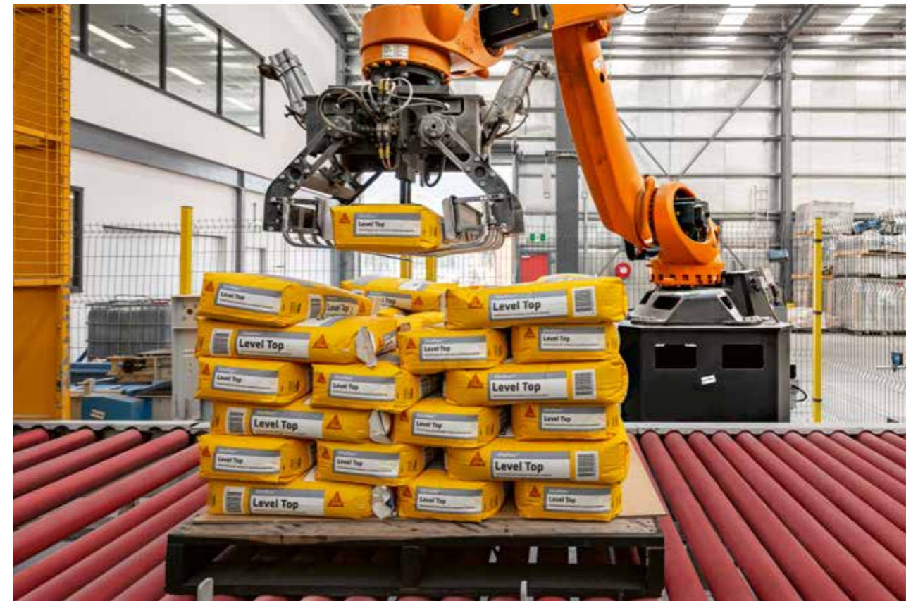
Robots prepare packed mortar for onward transportation. The fully automated procedures lower production costs.
