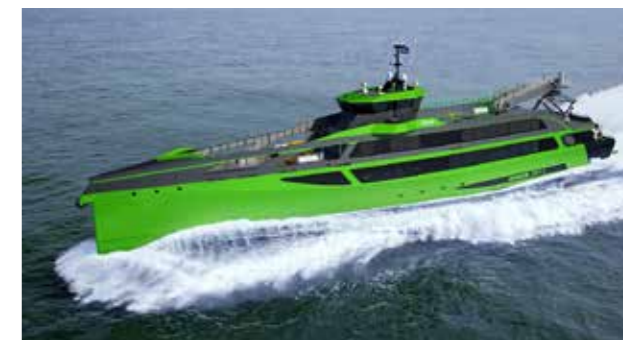
Damen Shipyards' new Fast Crew Supplier FCS-7011 is its latest development in the offshore crew fast-transfer sector. Sika is working together with the Damen Shipyards RGD team with a special emphasis on sealants, window and structural bonding. Sika provides all sealing and bonding materials, leading to a tremendous reduction in weight, faster total speed of application, and a decrease in building costs. In addition, Sikafloor® Marine decorative resins are included in the sanitary units creating perfect watertight floor compartments.
