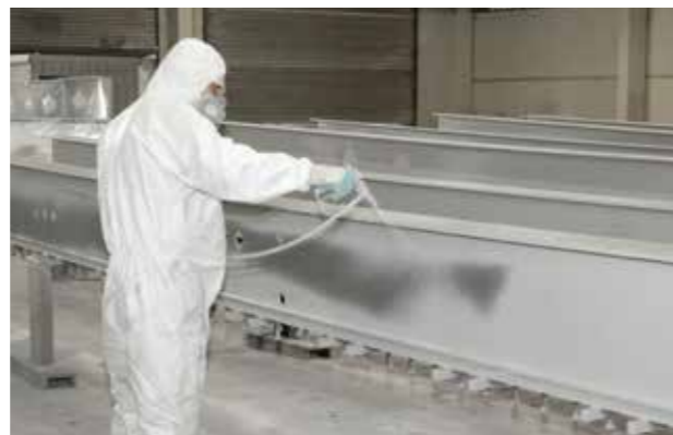
Sika's Platinum technology can be applied directly at the manufacturer's and is ready for transportation and assembly only 24 hours later. In the picture: Schneider + Co GmbH.
