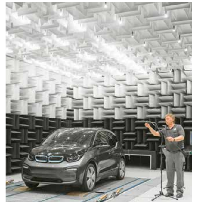
Quality you can hear. Testing solutions for reducing structure-borne noise in the BMW i3 at the acoustics center in Worms.
