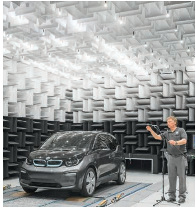
Quality you can hear. Testing solutions for reducing structure-borne noise in the BMW i3 at the acoustics center in Worms.
