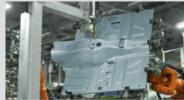
More safety, less weight, optimum stiffness: the innovative adhesive enables the body structure to absorb more energy.
